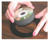
**Note:** It is important to not move the drum when placing the ring over it. Use both hands: reach one hand through the ring to hold the drum in place while pushing the ring down over the drum with the other hand. Subsequently hold the ring in place while lifting the drum away with the other hand.
