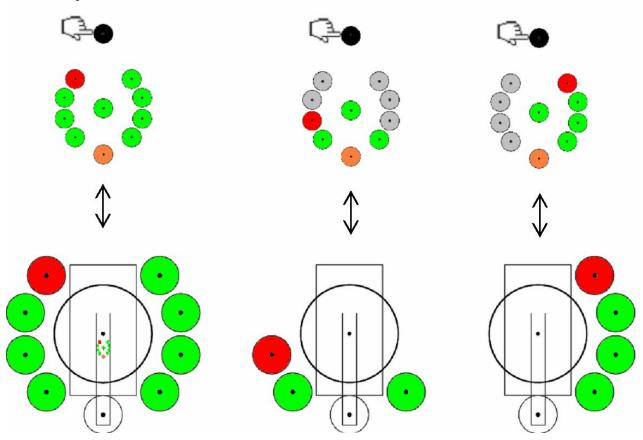
**Note**: The bins represented in green are filled with blank discs. The red one must be empty.
