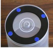
The bottom of the bins ("cake boxes") must mate nicely with the bin-supporting rings, which are 121mm diameter. The bottom of the bin should look like the one in the picture.
