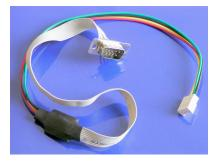
This electronic module/cable assembly is the interface between the Wytron controller and robot. The DB9 (RS232) connector should be installed at the rear of the tower, while the other end should be connected to the controller's COM2 port.
