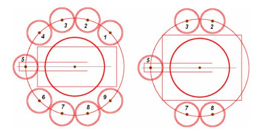
With the command set provided, each location may be either a disc bin or a processing unit tray. When controlling Dexterix from such a customized application, if not all 8 possible bin locations are required the master equipment may be wider than a regular disc duplication tower case. (The right side figure above shows an example where locations 1,4,6 and 9 are not used) Please see the "Dexterix' Developer's sheet" for details about controlling the robot externally, for custom applications.
