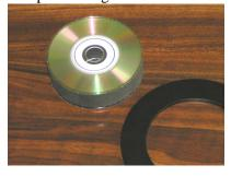
This 8cm diameter device is used during the interactive bin positioning procedure. The robot picks it from an open drive-tray and delivers it precisely to the location where the bin is to be positioned.
